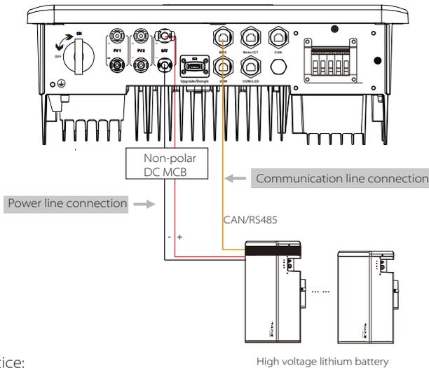
Notice: When using SolaX batteries, it is recommended that the number of battery control (T-BAT-5.8) is 1 and the number of battery modules (HV11550) is 0-2; the number of battery control (MC0600) is 1 and the number of battery modules (HV10230) is 1-4 pcs.
