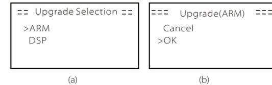
**Step 4.** Please confirm the new firmware version again and select the firmware to upgrade. The upgrade takes about 20 seconds. (d) When it is completed, the LCD screen returns to the "Update" page.
