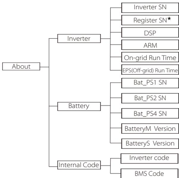
★ Register1 SN: Represents the serial number of external monitoring equipment, such as Pocket WiFi, Pocket LAN and Pocket GPRS.
