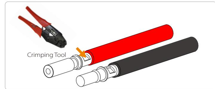
**Step 5.** The PV joint is divided into 2 parts - the plug and the fastening head. Insert the cable through the fastening head and the opposite plug. Notice that the red and black lines correspond to different of plugs. Finally, force the cable pair into the plug, will a "click" sound, which indicates that the connection is complete.
