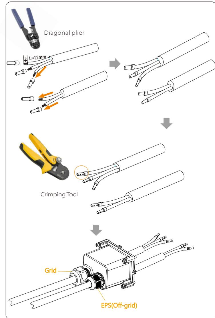
**Step 4.** Find the location of the AC interface on the inverter, insert the crimped terminals into the UW10 terminals L, N, and P according to the wire sequence, and use a flat-blade screwdriver to tighten the screws. (Torque:  $0.2 \pm 0.1 \text{ N} \cdot \text{m}$ )
