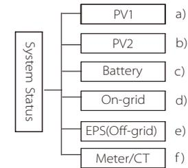
System status contains six content: PV1/PV2/Battery/On-grid (energy feed into or buy from the grid) and EPS(Off-grid) and so on. Press up and down to select, press "Enter" to confirm the selection, and press "ESC" to return to the menu.
