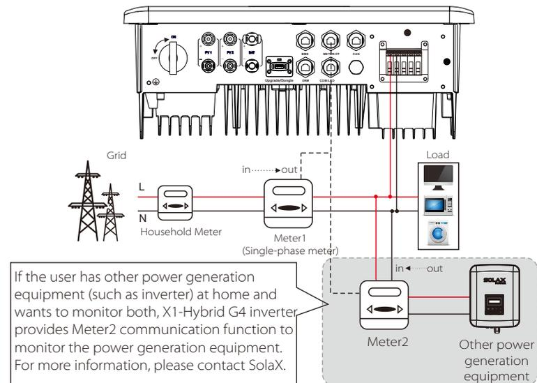
If the user has other power generation equipment (such as inverter) at home and wants to monitor both, X1-Hybrid G4 inverter provides Meter2 communication function to monitor the power generation equipment. For more information, please contact SolaX.
