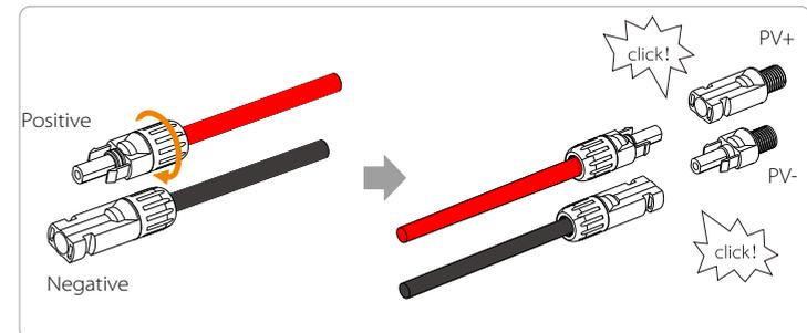
The following is the location of the inverter positive and negative (PV-/PV+) ports.
