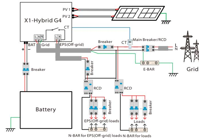
Diagram D: Neutral line and PE line are combined together, all loads connect to the EPS(Off-grid) port; (Apply to Australia)
