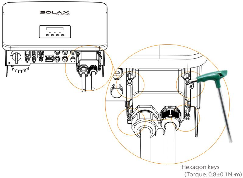
**Step 6.** Tighten the waterproof fastening head.
