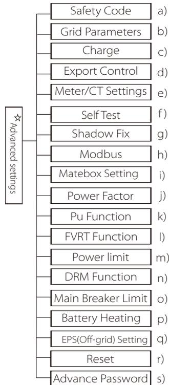
All advanced settings can be set here, such as battery, grid, EPS(Off-grid), etc.. "Advanced" setting is generally customization and resetting for battery and grid. Each part has lower level parts. Please contact your installer or factory and enter the installer password.
