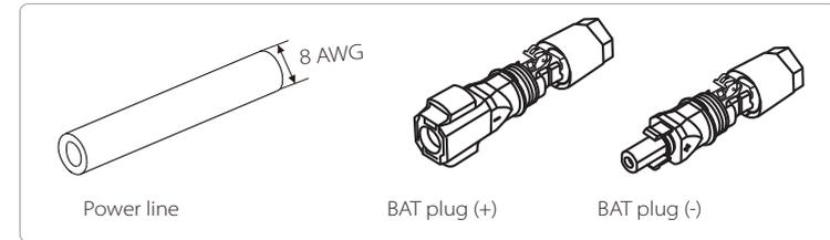
Step 2. Strip the insulation layer (length:15mm) at one end of the power line.
