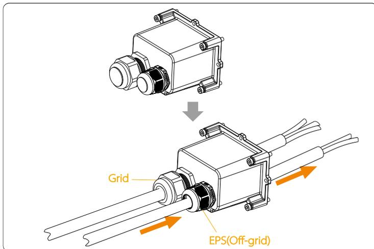
**Step 3.** Remove the 12mm insulation layer at the end of the wire. Insert the European-style terminals respectively, and make sure that the stripped ends are inserted into the European-style terminal, and finally use crimping pliers to press tightly.
