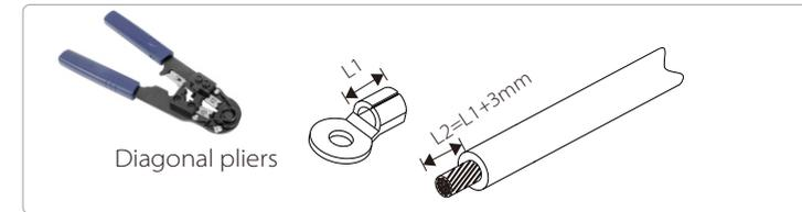
**Step 3.** Insert the stripped cable into OT terminal and tighten the terminal with a terminal crimping tool.
