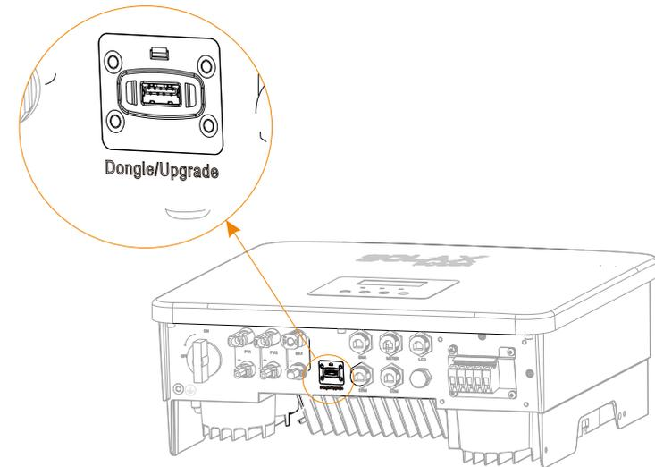
Step 2. Plug Pocket WiFi into the DONGLE port.
