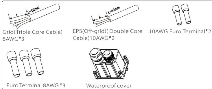
**Step 2:** The Grid and EPS(Off-grid) cables go through the corresponding Grid and EPS(Off-grid) ports of the waterproof cover.
