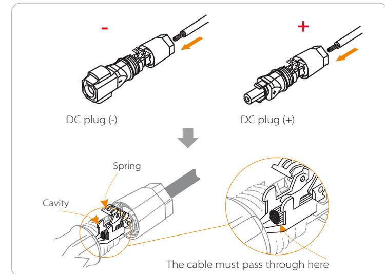
**Step 4.** Press down on the spring by hand, you can hear a click sound, then push the ends together, and tighten the screw joints.
