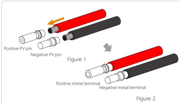
**Step 4.** Tighten the PV pin needle and the wiring harness to make the connection tight without looseness
