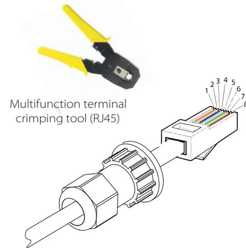
Multifunction terminal crimping tool (RJ45)
