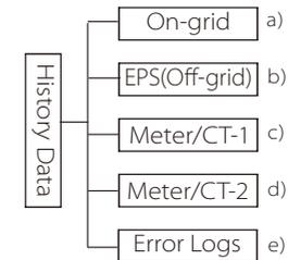
The history data contains five pieces of information: on-grid power of the inverter, EPS(Off-grid) power generation, power of the meter/CT and error logs.
