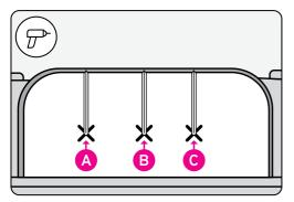
Secure the zappi to the structure using appropriate fixings, ensuring that the provided sealing washers (A) are used with all fixings (B) to maintain the IP rating.
