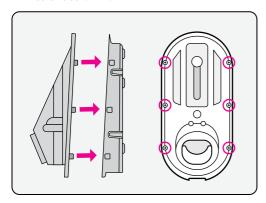
Refit the enclosure assembly ensuring clips on both sides make a positive fit to the back box.
