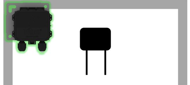
TAP attaches to module frame using built-in bracket. Mounting holes are also available in case of frameless modules.
