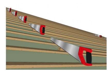
Cut upper batten flush with outside edge of panels, (this can be done after panels have been fitted)
