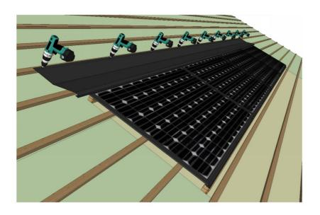
Fit top flashings securing using clips provided or tech screws
