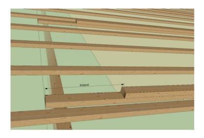
Single batten spanning from outside edge of array to supporting rafter if required.
