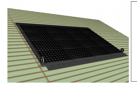
• Fit expandable foam tape to LHS & RHS flashing.
