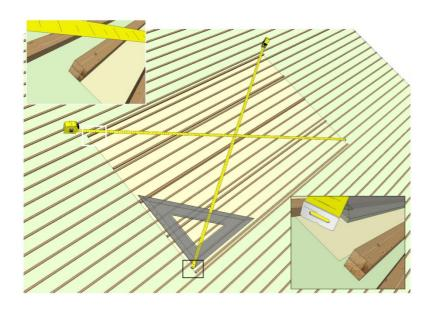
Make sure array panel mounting battens are square with the roof
