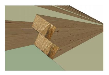
If / when horizontal supporting battens hits edge the existing batten. Span the joint with the upper batten and secure with screws
