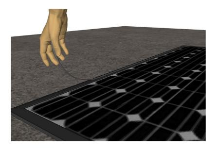
Remove top seal from panels for on top panel row to allow top flashing to be fitted
