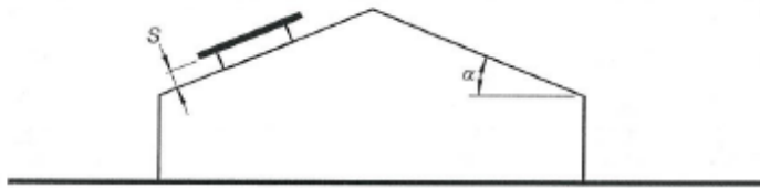
FIGURE D8 PANEL MOUNTED PARALLEL TO ROOF PLANE
