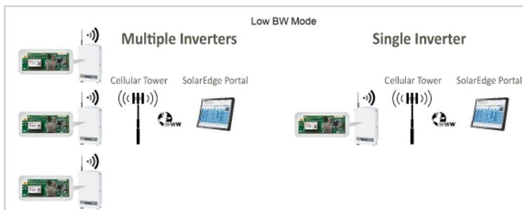
**Figure 1: GSM modem low BW mode connection diagram**
