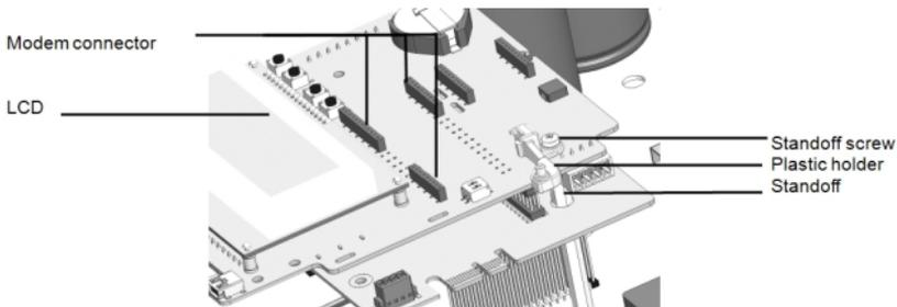
**Figure 11: The holder installed on the communication board**
