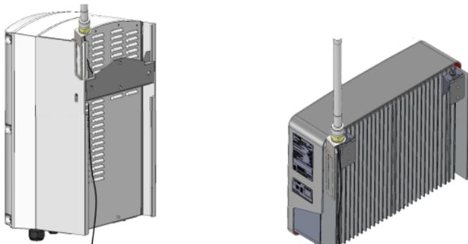
**Figure 6: Routing the antenna cable**
