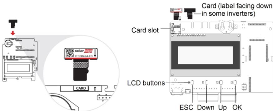
Figure 4: Communication board and activation card
