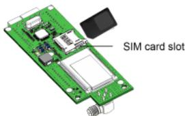
**Figure 9: Inserting the card into the GSM modem**
