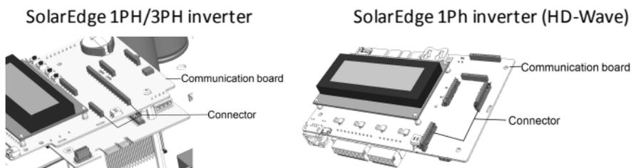
Figure 3: Communication board with GSM connector
