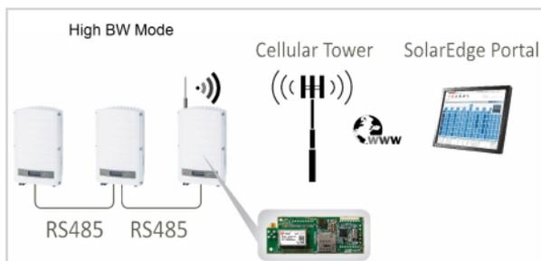
**Figure 2: GSM modem high BW mode connection diagram**
