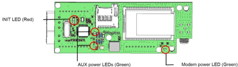
**Figure 14: GSM modem LEDs**
