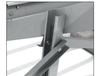
Fig.9 – Braces fit both sides of upright
