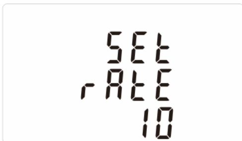
(It shows 1 impulse = 10kWh/kVArh)
