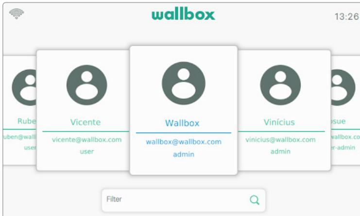
If multiple users are authorized to use the charger the login screen will show all the authorized users. Scroll to the sides to find and select the user. Use the Filter feature to speed up the search of users. Once selected, the PIN code of the user will be requested.
