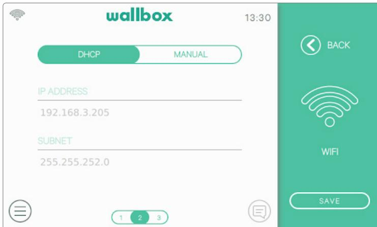
The network parameters are obtained automatically from the network's DHCP server and can be entered manually.
